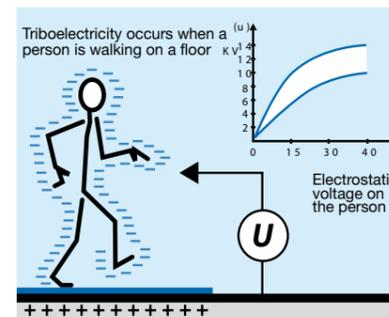
UCRETE® antistatic floors work by dissipating static electricity to earth. In order to prevent personnel working in the area from becoming charged through induction or triboelectrically, personnel must be in electrical contact with the floor, which requires the wearing of antistatic footwear.
